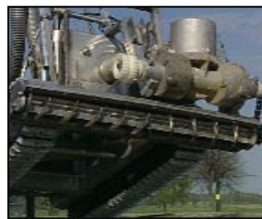
The YT-800 suction nozzle is vertically adjustable. The rotating screw chews up algae and sand without causing turbidity.
