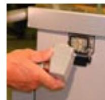
The floating cable is connected to the transformer by a plug and socket. This makes transportation and service easy and prevents the hose from twisting.
