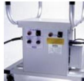
Transport trolley is equipped with transformer, timer radio control unit and sturdy lockable wheels.
