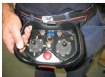
The YT-800 is equipped with a radio handbox that enables the operator to control all of the functions of the YT-800 from a distance. Together with the optional onboard cameras this means the operator can control the YT-800 from inside the operating room.
