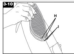
To replace the filter grill, insert tabs (H) at the bottom of the grill into slots (I) in the cleaner body. Press on grill to snap it into position.
