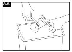
Brush the surface of filter to remove any clinging litter. (Filter may be washed in warm water. It must be **completely dry** before replacing in cleaner. **Do not use cleaner without filter in place.)**
