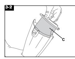
Hold cup over trash can. Remove filter (C) from top of cup.
