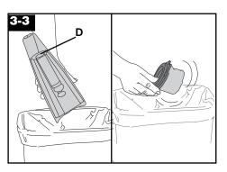
Empty cup, making sure to hold cup with dirt port (D) facing up. Shake dust from filter.
