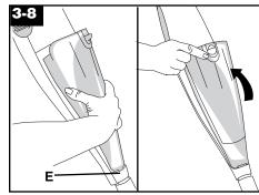
Place bottom of cup (E) first, then pivot cup into position. Press top of cup to snap it into place.
