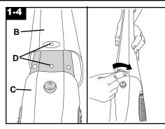
Push handle section (B) onto cleaner body (C), with holes (D) aligned. Insert toggle bolt through both holes and tighten by turning clockwise.
