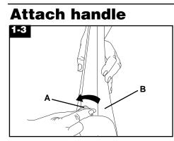
Remove the toggle bolt (A) from the handle section (B) by turning in a counterclockwise direction.
