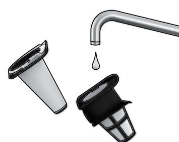
**4b.Separate both filters.** Dust container and filters can be shaken clean or rinsed in warm water (never in dishwasher). All parts must be dry before reassembled in reverse order.
