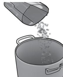
**2. Emptying of the dust container.** Remove the filters, empty the contents into a dustbin. Return filters and click dust container back into place.
