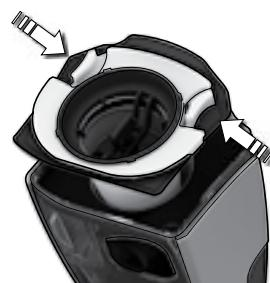
**4a.Cleaning of dust container and filters.** (Recommended every 5th cleaning). Release dust container, take out both filters by pressing release buttons.
