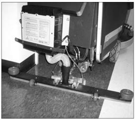
The unique breakaway squeegee assembly on the Wrangler 2016 keeps the machine working when others must be taken off the job to be repaired. If the assembly is inadvertently caught on a fixture or doorway, it releases from the holding bracket at the rear of the machine without bending or breaking. The assembly can be easily re-installed by simply hand tightening two control knobs.
