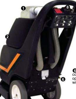
The twist-lock connector prevents the cord from accidently being pulled out.
