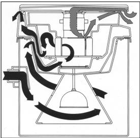
To quiet motor noise, suction air (black arrows) is squeezed through narrow openings and released into larger chambers within the powerhead—much like a car's muffler. A separate stream of clean, fresh air (gray arrows) cools the motor, protecting it from moisture and debris.
