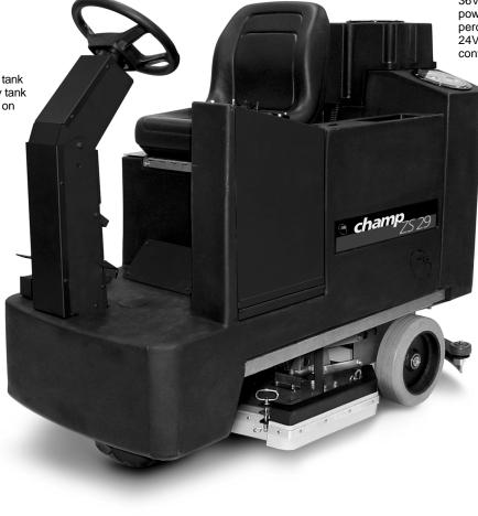
The flip-up battery cover allows easy access to the 36V. electrical system. This powerplant will generate 30 percent more run time than a 24V. system on a similarly configured unit.
