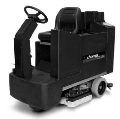
**The New Little Ride-On With 'Oomph.'** The new Champ 2929 from NSS<sup>®</sup> is the snappy little ride-on with big ride-on power. Its 36V. electrical system package delivers up to 30 percent more run time than a comparably configured 24V. machine, so the Champ 2929 gives you more of what you expect from a ride-on autoscrubber.
