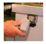
The floating cable is connected to the transformer by a plug and socket. This makes transportation and service easy and prevents the floating cable from twisting.
