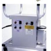
Transport trolley equipped with transformer, timer, radio control unit and sturdy lockable wheels.
