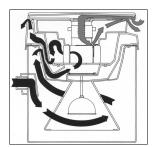
To quiet motor noise, suction air (black arrows) is squeezed through narrow openings and released into larger chambers within the powerhead—much like a car's muffler. A separate stream of clean, fresh air (gray arrows) cools the motor, protecting it from moisture and debris.
