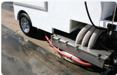
CYCLONE cleaning head both deep cleans and recovers water
