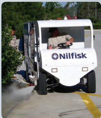
Kerb cleaner cleans the vertical face of the kerb
